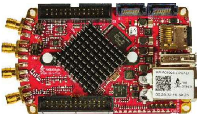
PHOTO 2: Modern test equipment such as the Red Pitaya (reviewed in October 2018) can make many measurements like PEP automatically.
