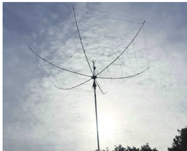
The hex beam was assembled and mounted on a rotator and portable mast.
