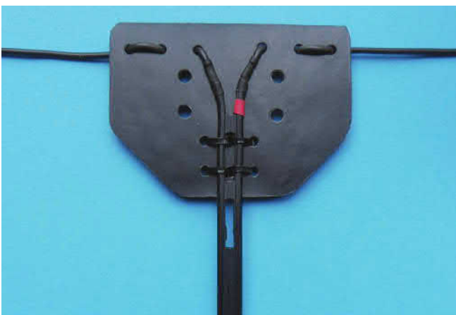
PHOTO 2: The doublet's dipole centre made from a sheet of uPVC.
